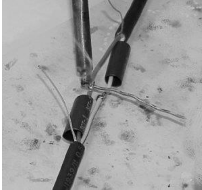
Solder Wires Together
