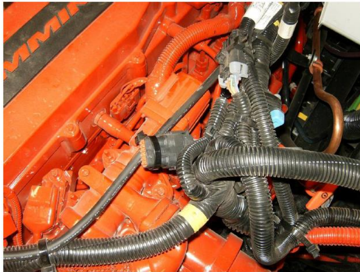
12-Way Connector (7207M) Center of Picture
